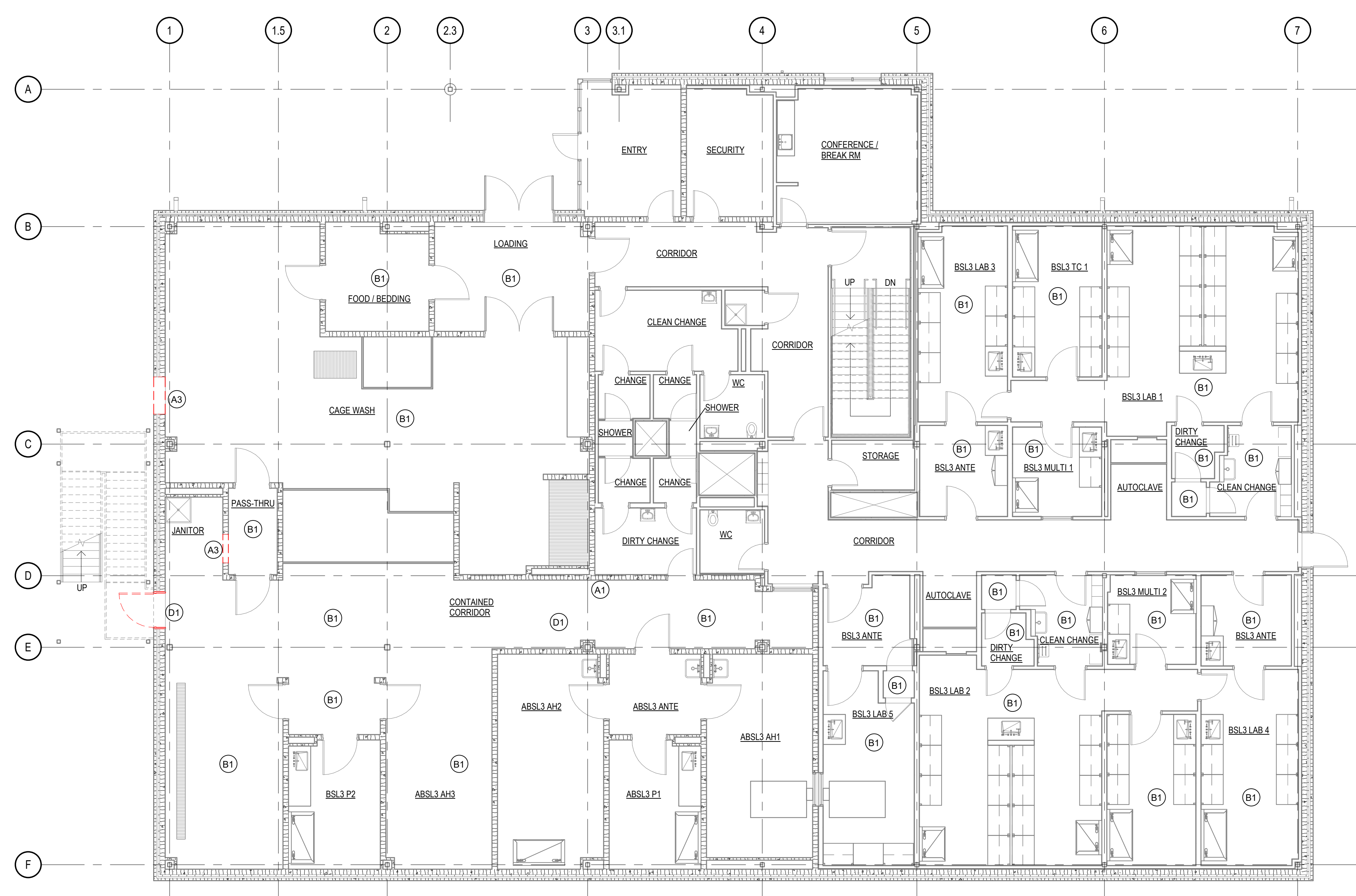
1 FIRST FLOOR DEMOLITION PLAN SCALE: 1/8" = 1'-0"
